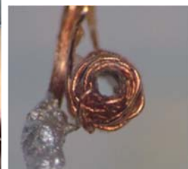
Mutual-inductance micro coil: 0.3 mm ID/1.0 mm OD.
