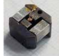
Fig. 1 Thermal contraction strain cell (9 x 9 x 5 mm 3 ).
